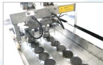
清洗后检验 Inspection after cleaning
